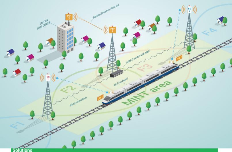
**Redundancy and** route optimization MINT protocol has the capability to work with multiple redundant paths, to optimize data flow using all available connections from one customer point to another. IW recommends the use of at least two CPEs in order to have two different paths to deliver customer traffic. Path selection and traffic flow switches between paths handled by the unique IW transport protocol MINT.
