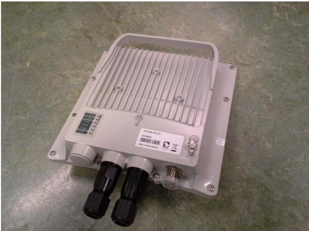
**Picture 8:** EUT type InfiLINK XG Um. External antenna 28 dBi, 4.9-6.425 GHz Band
