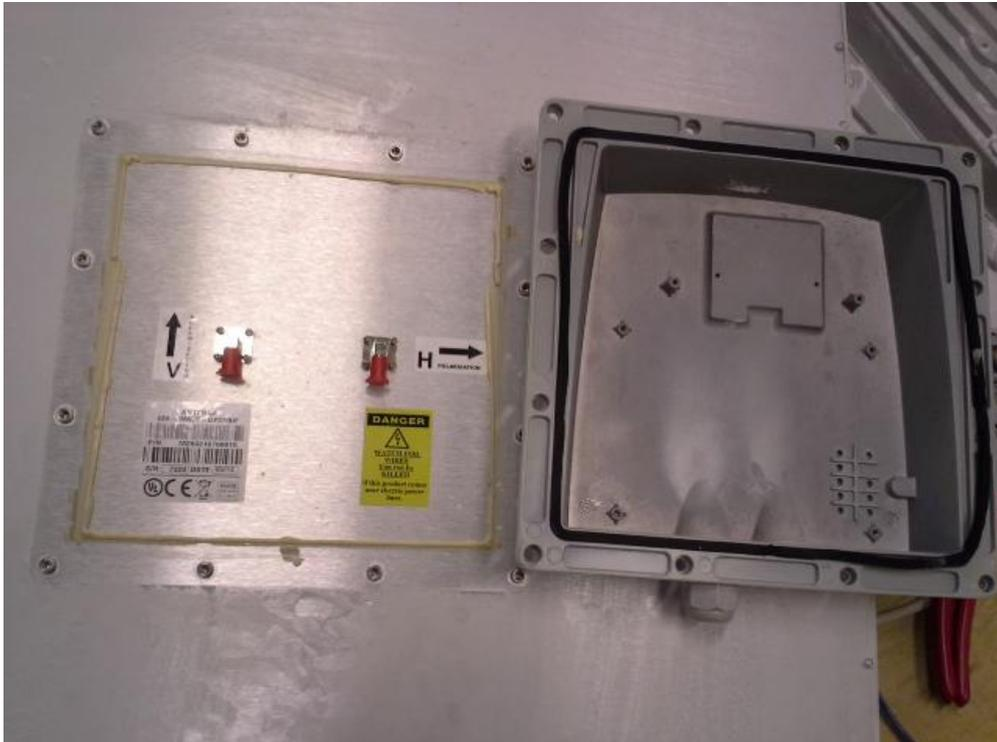
**Picture 31:** EUT R5000-Smn. Antenna 28 dBi, 4.9-6.425 GHz Band.
