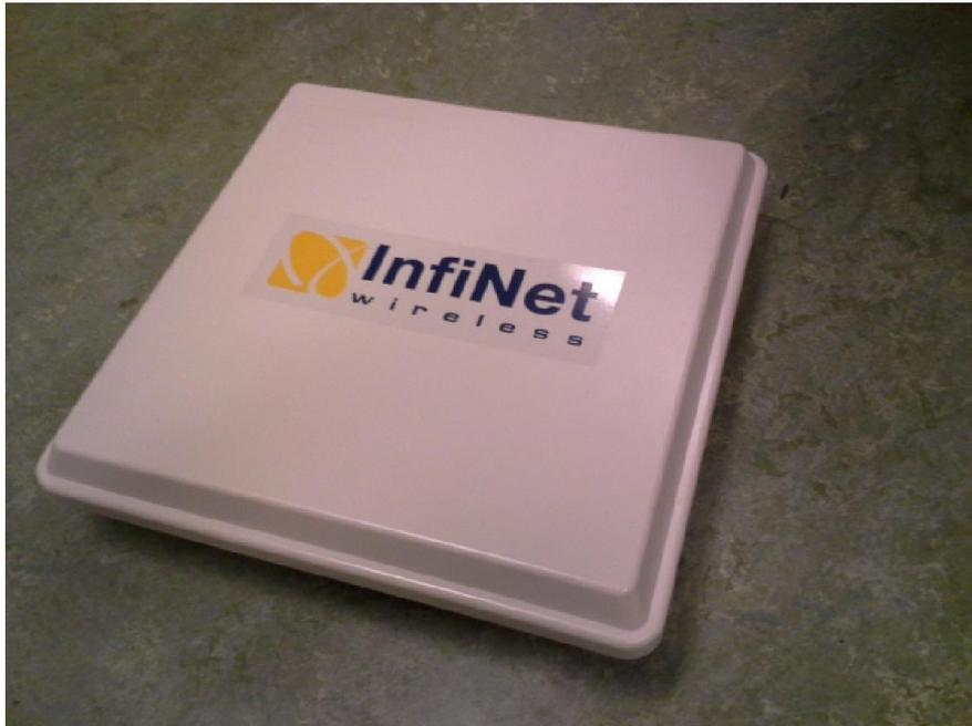
**Picture 1:** EUT type R5000-Mmx. Antenna 23 dBi, 3.4-6.425 GHz Band
