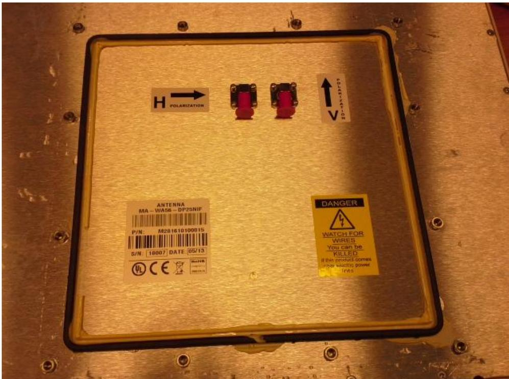
Picture 24: EUT type R5000-Mmx. Antenna 23 dBi, 3.4-6.425 GHz Band. No trace of water inside the enclosure after the IPX7 test
