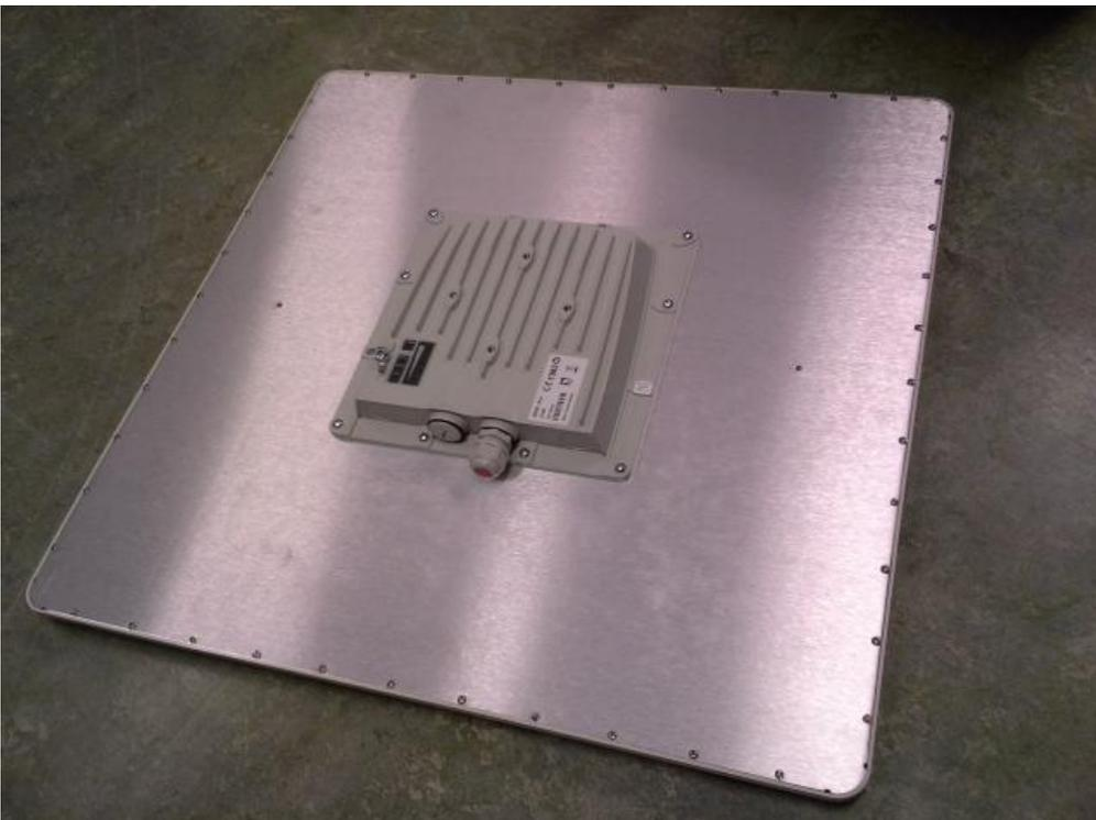
**Picture 14:** EUT R5000-Smn. Antenna 28 dBi, 4.9-6.425 GHz Band
