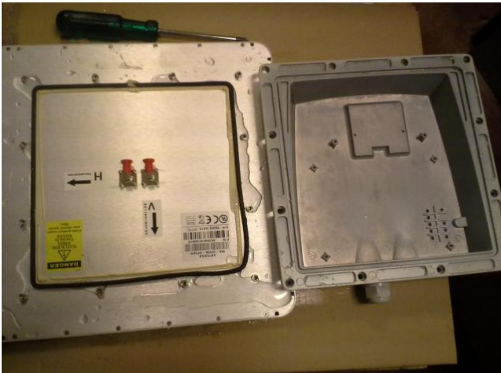
**Picture 30:** EUT R5000-Smn. Antenna 21 dBi, 4.9-6.425 GHz Band.
