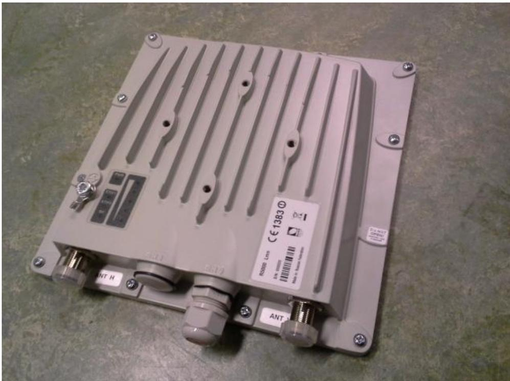
**Picture 16:** EUT R5000-Lmn. External antenna, 3.4-6.425 GHz
