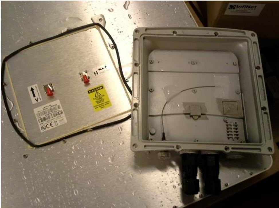
**Picture 27:** EUT type InfiLINK XG Xm. Antenna 28 dBi, 4.9-6.425 GHz Band. No trace of water or dust inside the enclosure after the IP6X, IPX6 and IPX7 tests.
