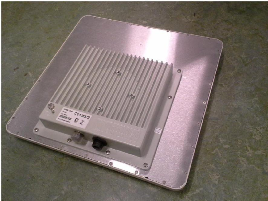
**Picture 2:** EUT type R5000-Mmx. Antenna 23 dBi, 3.4-6.425 GHz Band
