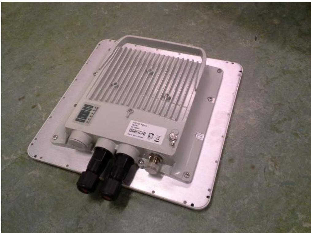
**Picture 4:** EUT type InfiLINK XG Xm. Antenna 23 dBi, 4.9-6.425 GHz Band
