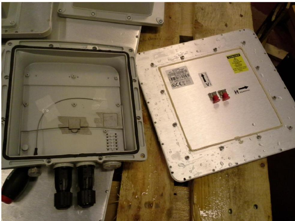
**Picture 26:** EUT type InfiLINK XG Xm. Antenna 23 dBi, 4.9-6.425 GHz Band.
